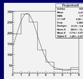
Projected charge (in units of photoelectrons) released by a 140 keV simulated γ fitted with a Gaussian distribution superimposed on a flat background
