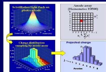
Schematic illustration of Sampling Procedure
