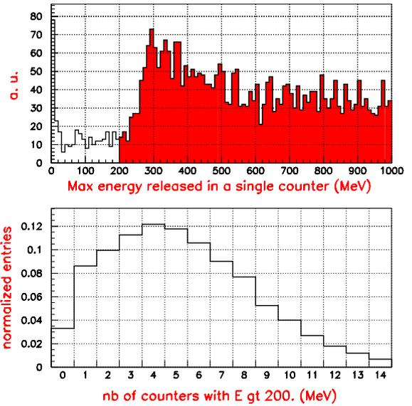
Fig. 8. Top: maximum energy loss in a single scintillation counter by internal  $\nu_\mu$  CC interactions. Bottom: number of counters with an energy release greater than 200 MeV.
