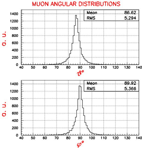
Fig. 3. Zenithal (top) and azimuthal (bottom) angle distributions of  $CNGS$   $\mu$  in the LVD reference system:  $\theta = 90^\circ \equiv$  horizontal;  $\phi = 90^\circ \equiv$  parallel to the Hall A-axis.
