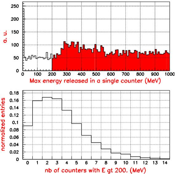
Fig. 9. Top: maximum energy loss in a single scintillation counter by internal  $\nu_\mu$  NC interactions. Bottom: number of counters with an energy release greater than 200 MeV.
