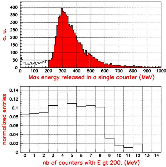
Fig. 7. Top: maximum energy loss in a single scintillation counter by a CNGS  $\mu$ . Bottom: number of scintillation counters with an energy release greater than 200 MeV.
