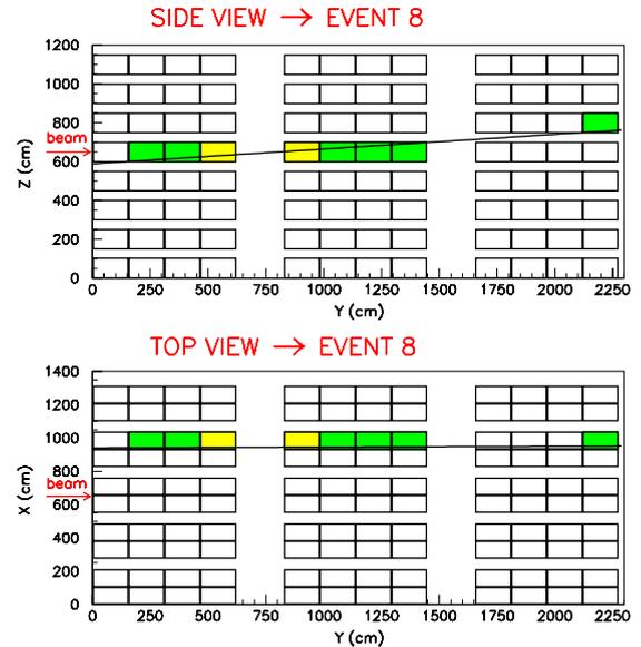
Fig. 5. Event display of a CNGS  $\mu$  crossing eight scintillator counters.
