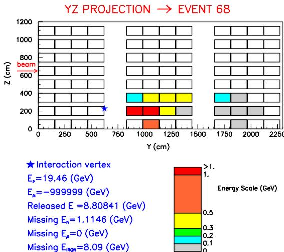
Fig. 11. Event display of CNGS  $\nu_\mu$  neutral current internal interaction.
