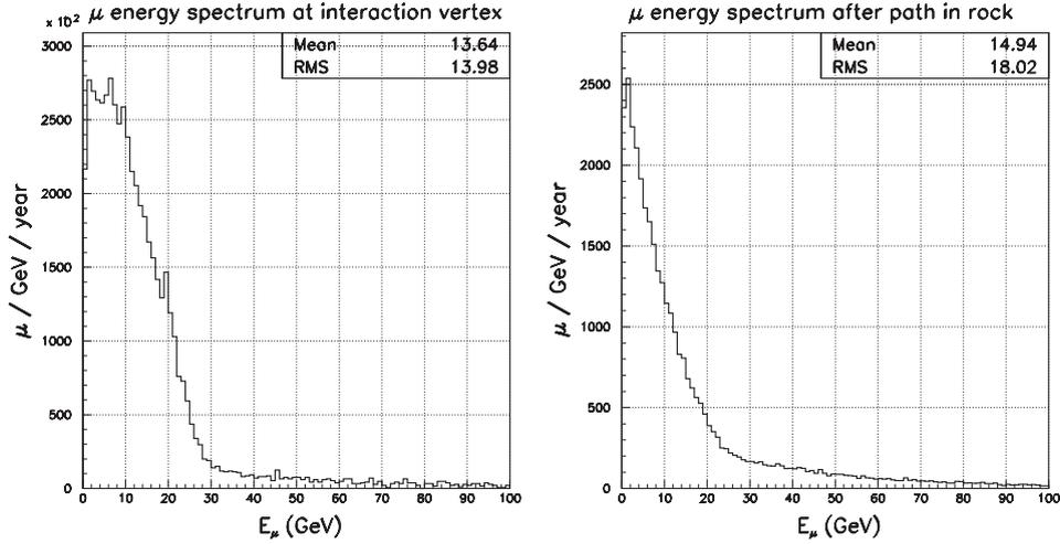
Fig. 2. Energy spectra of the  $\mu$  generated in charged current  $\nu_\mu$  interactions at the interaction vertex (left) and after path in rock, when entering the experimental hall (right).
