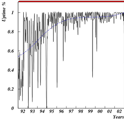
**Fig. 1.** Weekly averaged duty cycle in the LVD detector since June 1992.
