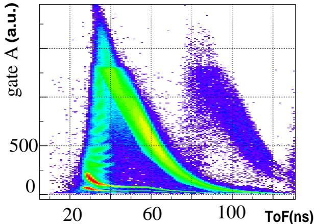
Fig. 1. Correlation plot of Short-gate integrated Light Output vs. ToF as seen from one of the Phoswiches.
