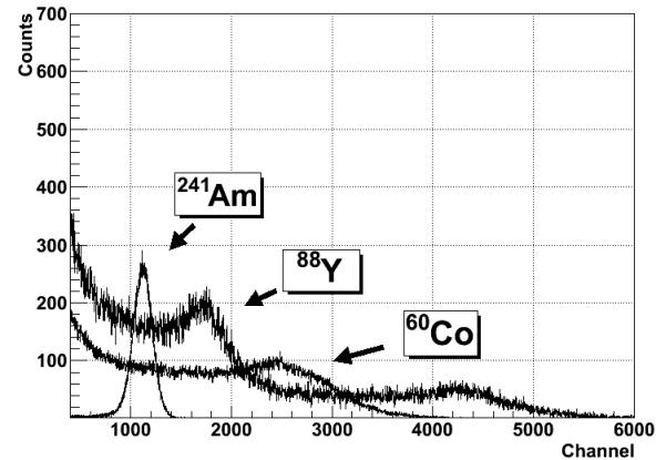
Fig. 2. Non normalized  $\alpha$  particle ( ${}^{241}\text{Am}$ ) and  $\gamma$  ray ( ${}^{88}\text{Y}$ ,  ${}^{60}\text{Co}$ ) spectra for the L1 sample.
