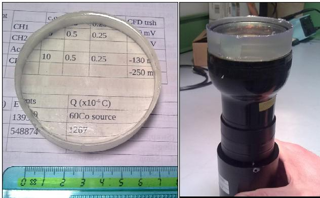
Fig. 1. Photo of the large volume siloxane scintillator produced (on the left) and of the same mounted on the PMT.
