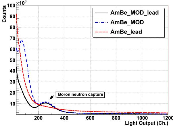
Fig. 3. Spectra from the AmBe source for the L2\_B3 sample: fast neutron spectrum obtained with Lead shielding on the detector (dashed line); partially moderated (through HDPE) neutron spectrum without lead shielding (dot-dashed line); partially moderated neutron spectrum with lead shielding.
