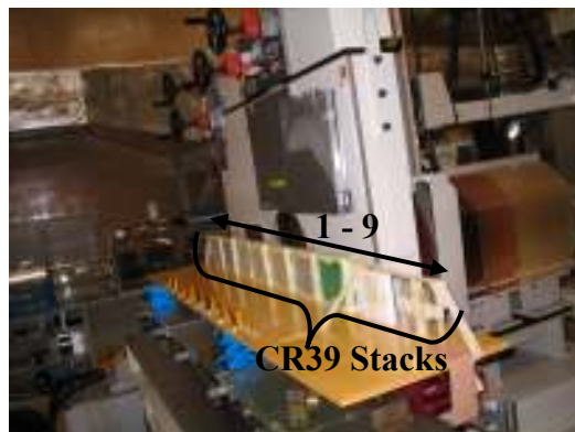
Fig. 4.5 Exposure set-up for the stacks of CR39 and Makrofol NTDs at HIMAC, Chiba, Japan.
