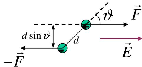
$$U_E = q\Delta V_+ - q\Delta V_- = -\frac{d}{2}Eq \cos \vartheta - \frac{d}{2}Eq \cos \vartheta$$
