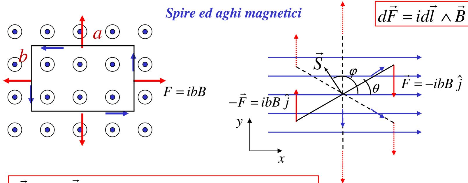
$$\begin{aligned} \vec{\mathcal{M}} &= \vec{a} \wedge \vec{F} \\ &= \vec{a} \wedge (-ibB \hat{j}) = -iBba (\cos \theta \hat{i} + \sin \theta \hat{j}) \wedge \hat{j} \\ &= -iSB \cos \theta \hat{k} = -iSB \sin \varphi \hat{k} = i\vec{S} \wedge \vec{B} \end{aligned}$$
