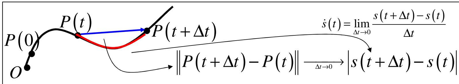
$$\|\vec{v}(t)\| = \lim_{\Delta t \rightarrow 0} \frac{\|P(t + \Delta t) - P(t)\|}{\Delta t} = \lim_{\Delta t \rightarrow 0} \frac{|s(t + \Delta t) - s(t)|}{\Delta t} = |\dot{s}(t)| = v(t)$$
