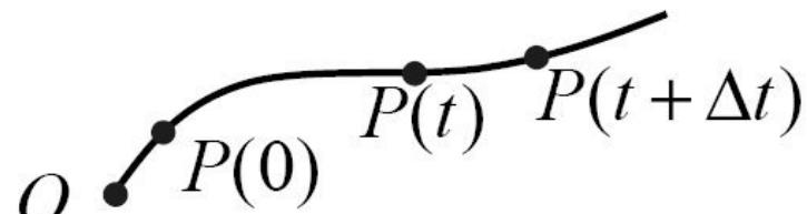
$$\begin{aligned}s_0 &= \widehat{OP}(0) \\ s(t) &= \widehat{OP}(t) \\ s(t + \Delta t) &= \widehat{OP}(t + \Delta t)\end{aligned}$$
