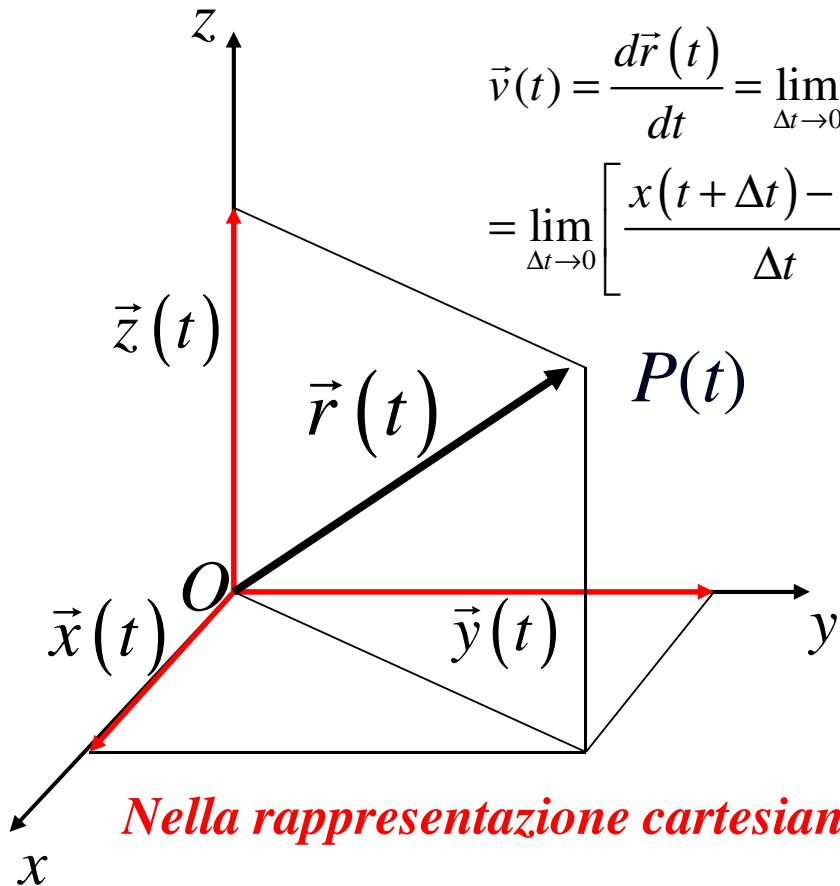
$$\begin{aligned}\vec{v}(t) &= \frac{d\vec{r}(t)}{dt} = \lim_{\Delta t \rightarrow 0} \frac{\vec{r}(t + \Delta t) - \vec{r}(t)}{\Delta t} \\ &= \lim_{\Delta t \rightarrow 0} \left[ \frac{x(t + \Delta t) - x(t)}{\Delta t} \hat{i} + \frac{y(t + \Delta t) - y(t)}{\Delta t} \hat{j} + \frac{z(t + \Delta t) - z(t)}{\Delta t} \hat{k} \right]\end{aligned}$$
