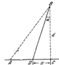
$$t(x) = \frac{s-x}{v_2} + \frac{\sqrt{x^2+d^2}}{v_1}$$
