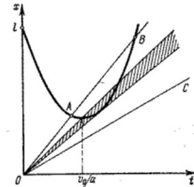
$$\left. \begin{aligned} s_A &= v_A t \\ s_B &= \frac{1}{2} a t^2 - v_0 t + l \end{aligned} \right\} v_A t_i = \frac{1}{2} a t_i^2 - v_0 t_i + l \Rightarrow a t_i^2 - 2(v_0 + v_A) t_i + 2l = 0$$
