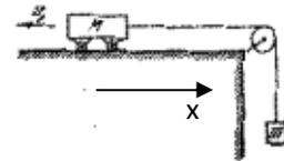
$$\left. \begin{aligned} T &= Ma \\ mg - T &= ma \end{aligned} \right\} ma = mg - Ma \Rightarrow a = \frac{m}{m + M} g = \frac{2}{7} 9.8 = 2.8 \text{ m/s}^2$$
