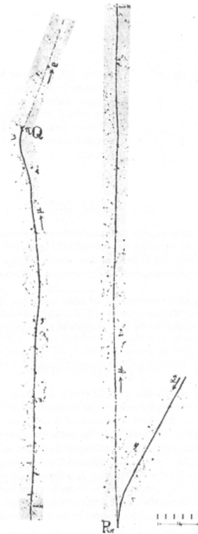
Figure 3.1: A \kappa ( K ) meson stops at P , decaying into a muon and neutrals. The muon decays at Q to an electron and neutrals. The muon track is shown in two long sections. Note the lighter ionization produced by the electron, contrasted with the heavy ionization produced by the muon near the end of its range. The mass of the \kappa was measured by scattering and grain density to be 562 \pm 70 \text{ MeV} (Ref. 3.4).
