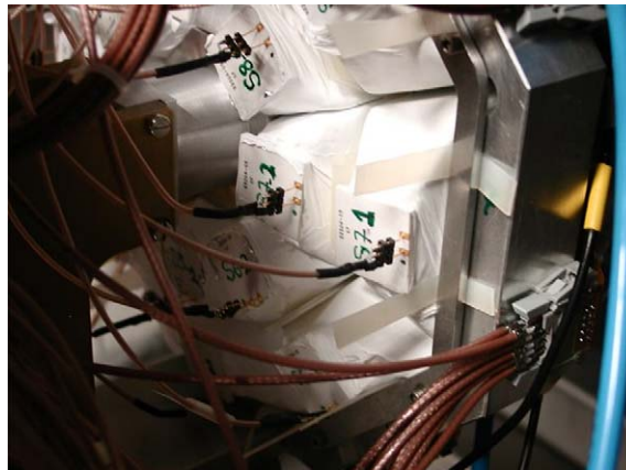
Fig. 3. Picture of the RCo detector from behind, showing the details of the CsI(Tl) crystals, mounted in the holder.
