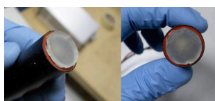
Fig.3: Coupling with Hamamatsu H6524 PMT.
