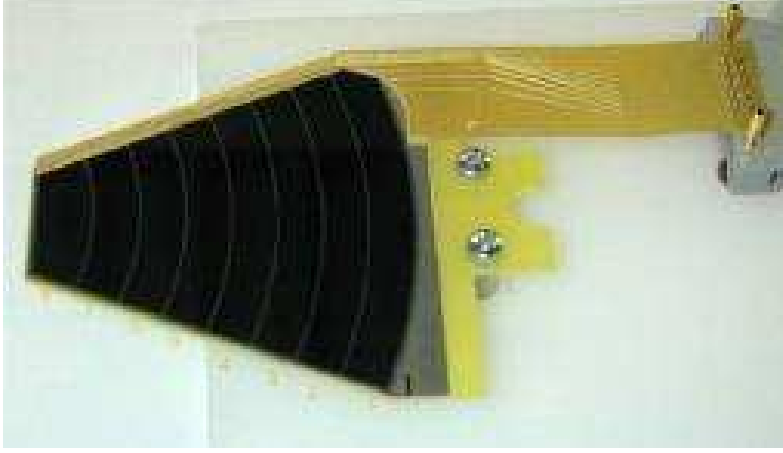
Figure 2.8: One of the Si detectors of the RCo. Each one of the eight strips has a size of 8.55 mm. The full length of the silicon detector is 68.4mm (see Table 1).
