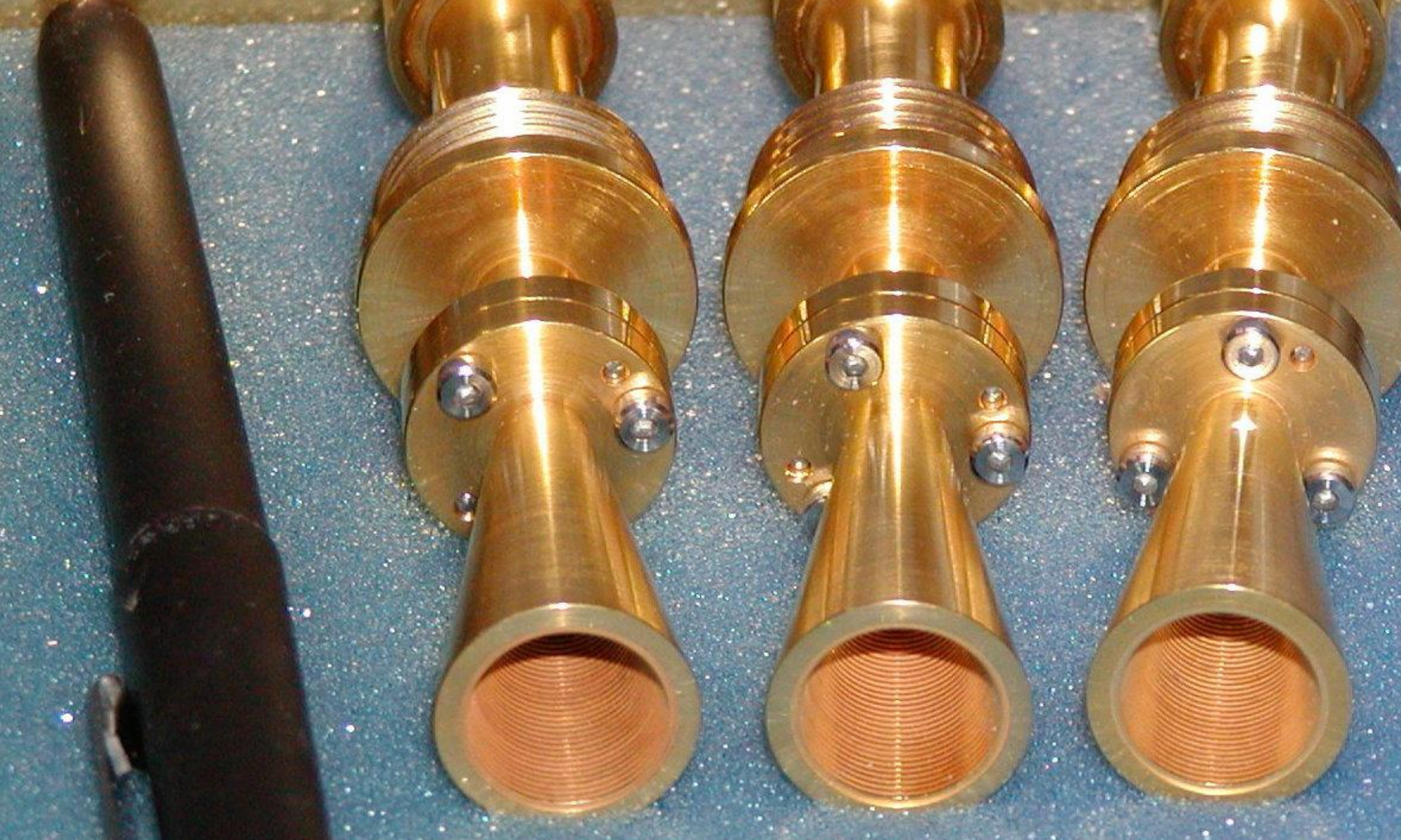
The Back to Back input feeds (150 GHz)
