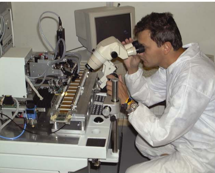
Bonding and inspection of ladders
