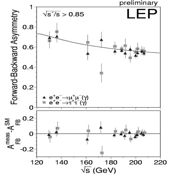
Figure 3. Preliminary combined LEP results on the forward-backward asymmetries for  $\mu^+\mu^-$  and  $\tau^+\tau^-$  final states as a function of centre of energy
