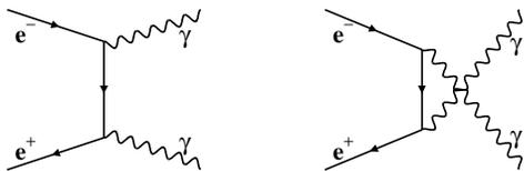
Figure 6. Lowest order diagrams for  $e^+e^- \rightarrow \gamma\gamma$
