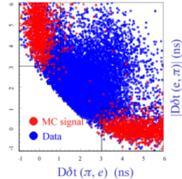
$\pi/e$  identification using time-of-flight
