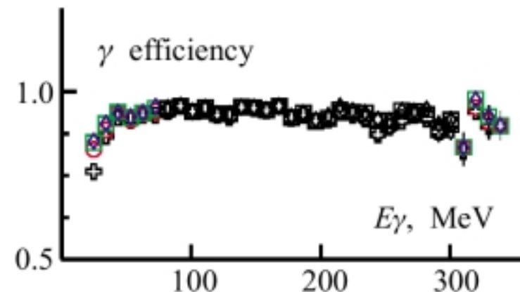
Trigger efficiency estimated by measuring probability of having 0,1 triggering clusters from data
