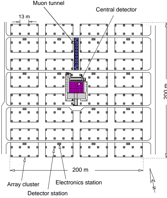
Figure 1. The KASCADE experiment near Karlsruhe. The array of 252 detector stations is subdivided into 16 clusters, each with a dedicated electronics station for data readout.
