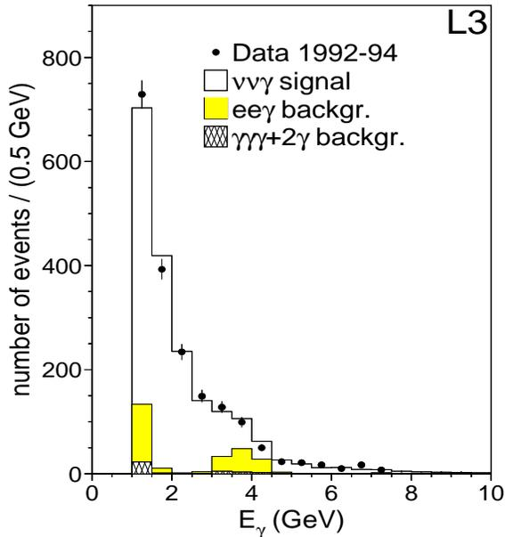
Figure 2. Energy spectrum of the single photons for data and Monte Carlo predictions [9,10] obtained by L3
