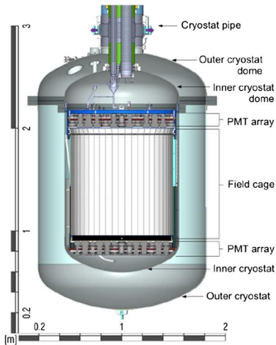
**Fig. 1** The XENON1T TPC with cryostat, section view, subgroups are indicated with reference to the “XENON1T Use” column of Table 1
