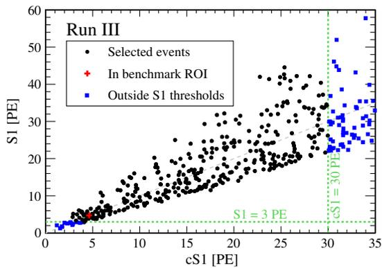
FIG. 3. The S1 and  $cS1$  derived from the LCE for the run III data. Events below the lower S1 threshold at  $S1 = 3 \text{ PE}$  (horizontal line) and above the upper threshold at 30 PE in  $cS1$  (vertical line) are removed from the analysis (blue squares). The  $S1 = cS1$  line is shown for reference. The dark matter candidate in the ROI is highlighted (red cross).
