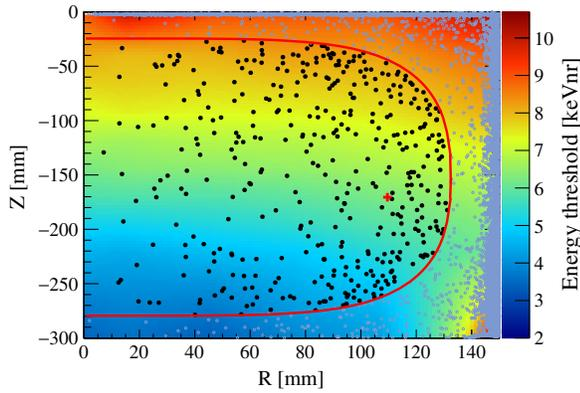
FIG. 2. The varying energy threshold in  $\text{keV}_{\text{nr}}$  due to the new threshold in S1, inside the active volume of the TPC as a function of the radius,  $R$ , and depth,  $Z$ . The color scale is a mapping of the LCE and  $S1 = 3 \text{ PE}$  to energy assuming average values of  $\mathcal{L}_{\text{eff}}$  and  $Q_y$ . The run III data inside (solid black points, with red cross for the candidate in the ROI) and outside (hollow gray points) the fiducial volume (red line) are shown.
