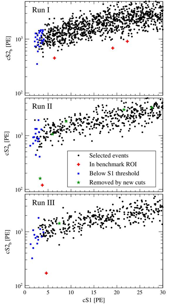
FIG. 1. The  $cS1$  and  $cS2_b$  for runs I (top), II (middle), and III (bottom) science data passing all selection criteria (black circles, with red crosses for dark matter candidates in the ROI). Events that fall below the S1 threshold (blue squares) are not used in the analysis. Events that were removed by the new high S1 rate and improved S2 classification cuts are also shown (green stars). The total number of events is summarized in Table I.
