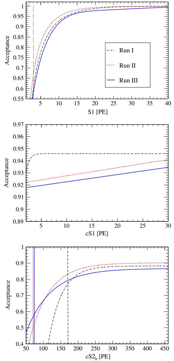
FIG. 4. The combined acceptance of the S1 coincidence cut and noise misidentification (top), and the cumulative acceptance of the rest of the  $cS1$ -based cuts (middle) and  $cS2$ -based cuts (bottom), for each science run. The acceptance in  $cS2$  is constant above 450 pe. The S2 thresholds for each run are indicated by the vertical lines.
