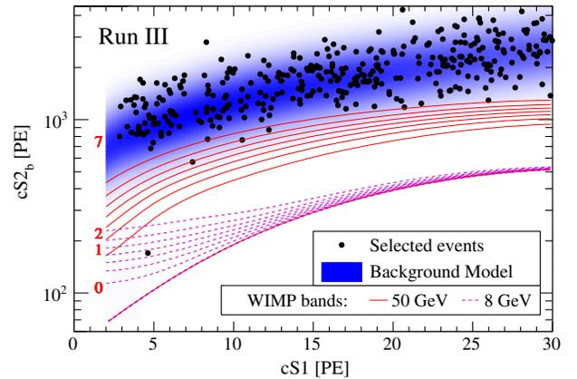
FIG. 5. Example bands for 8 GeV/ $c^2$  (purple dashed lines) and 50 GeV/ $c^2$  (red solid lines with numbered labels) WIMP mass SI signal models. The lower bound for all WIMP masses is defined by the 20 GeV/ $c^2$  model as described in the text. The upper bound of the topmost band is beyond the vertical range. The shape of the background model is shown with a (blue) linear color scale. The run III science data are overlaid for reference.
