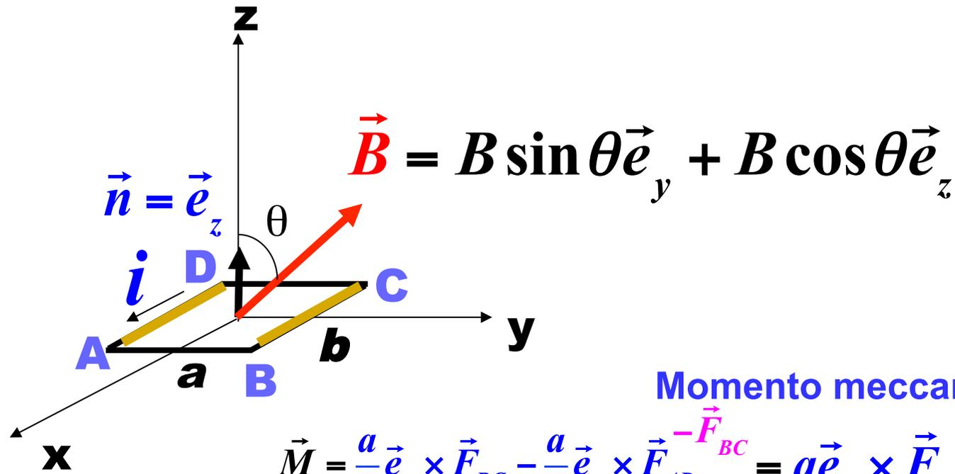
$$\begin{aligned} \vec{M} &= \frac{a}{2} \vec{e}_y \times \vec{F}_{BC} - \frac{a}{2} \vec{e}_y \times \vec{F}_{AD} = a \vec{e}_y \times \vec{F}_{BC} \\ &= a \vec{e}_y \times (-ibB \sin \theta \vec{e}_z + ibB \cos \theta \vec{e}_y) = -iabB \sin \theta \vec{e}_y \times \vec{e}_z \\ &= iabB \sin \theta \vec{e}_z \times \vec{e}_y = iA \vec{n} \times \vec{B} = \vec{m} \times \vec{B} \end{aligned}$$
