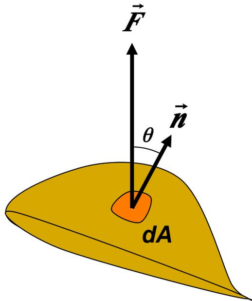
$$\Phi_{\Sigma}(\vec{F}) = \int_{\Sigma} d\Phi(\vec{F}) = \int_{\Sigma} \vec{F} \cdot \vec{n} dA$$
