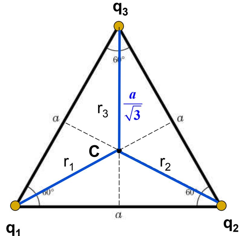
$$V_C = V_1 + V_2 + V_3 = \frac{1}{4\pi\epsilon_0} \left[ \frac{q_1}{r_1} + \frac{q_2}{r_2} + \frac{q_3}{r_3} \right] = \frac{\sqrt{3}}{4\pi\epsilon_0 a} (q_1 + q_2 + q_3)$$
