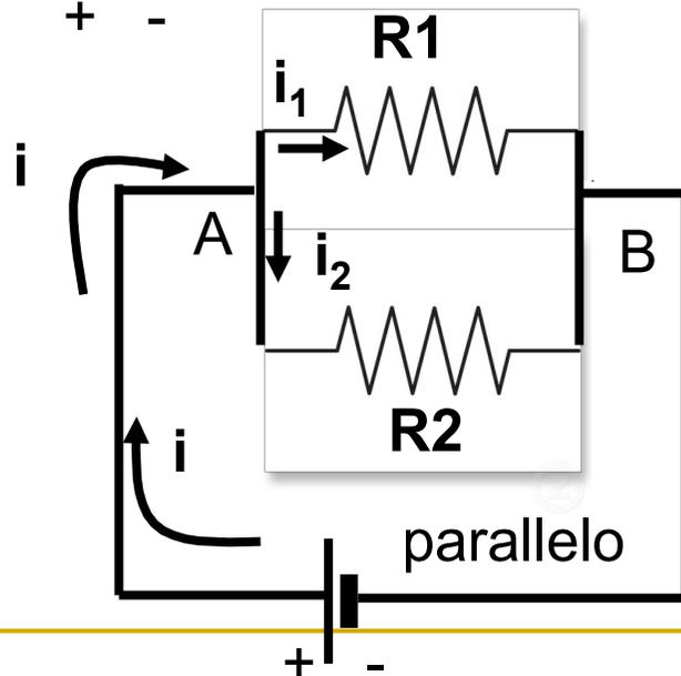
$$i = i_1 + i_2 = \frac{V}{R_1} + \frac{V}{R_2}$$
