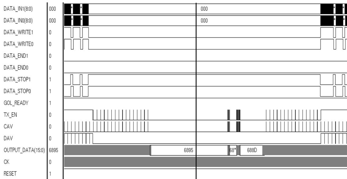
**Timing 13:** When CARLOSrx applies a back-pressure towards CARLOS, the *data\_stop* signals are asserted. Then, if desired, CARLOS can be put in JTAG mode and some JTAG operations can be performed (the reading of an internal register in figure). Then CARLOS can be put in RUN mode again and data acquisition process restarted.
