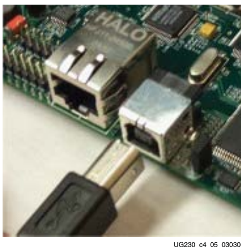
Figure 4-4: Connect the USB Type B Connector to the Starter Kit Board Connector
