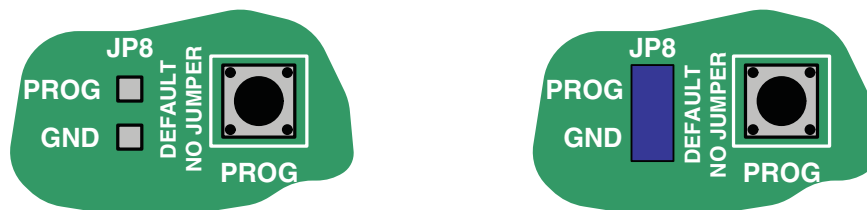
a) No Jumper: FPGA Operational (default)
